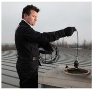
The most effective method of inspecting things such as chimney and downpipes is from above. For example when standing on the roof. To do so, it is necessary to connect a camera cable to the monitor.
