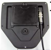
Fig. 9: Camera cable fed through guide
