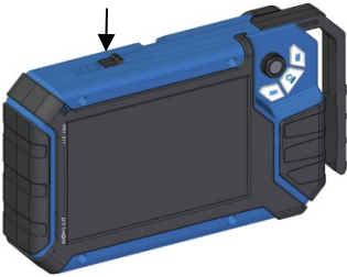
Fig. 17: Push button for pulling out the handle marked with arrow
