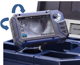
Fig. 13: You can turn and tilt the monitor
