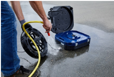
Fig. 68: Cleaning the viper and the rod
