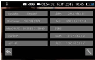
Fig. 45: Info menu with SOM (Firmware of the camera) and CAM (Version of the camera head)
