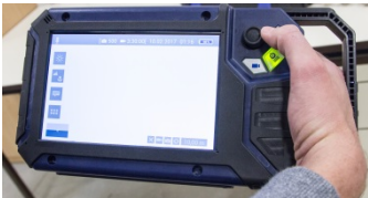
Fig. 16: With the handle pulled out it is possible to hold and operate the monitor with one hand.
