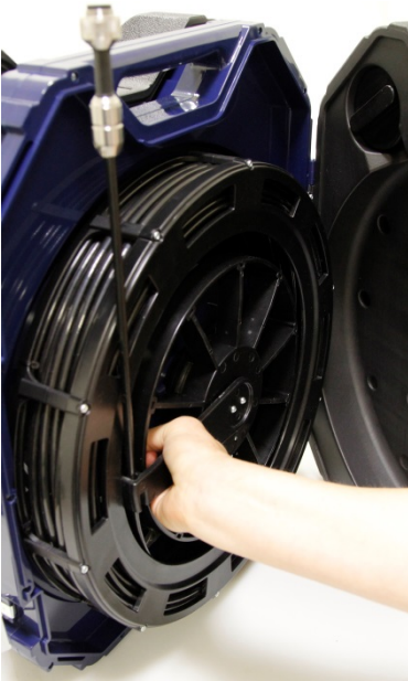
Fig. 65: Grasping the end of the rod and the viper
