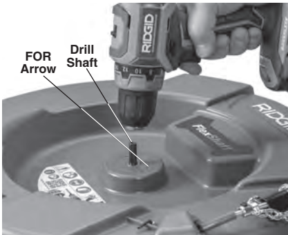
Figure 4 – Attaching Drill To Drill Shaft
