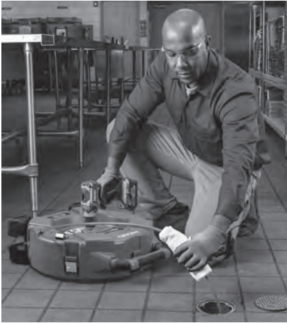
Figure 13 – Applying Lubricant to the Cable Sheath
