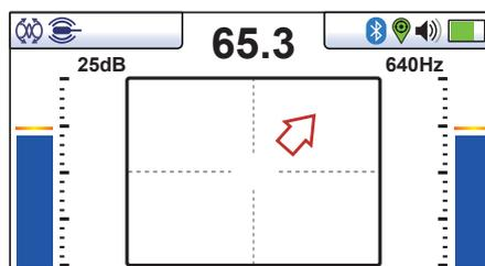
6. If the bar graph is not steady it will most likely be because the sonde is not within range. In this case hold the locator at approximately 45 degrees to the ground and rotate the locator around a full 360 degrees around you. Note the direction of strongest signal and walk towards it until the bar graph shows a steady signal. Now revert to step five above.
