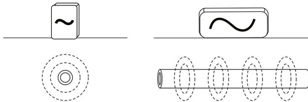
Remove any connections from the output connector. Switch on the transmitter and place it over the suspected position of the line and position it so that it is in line of the target as above. In the case of the Loc3-10Tx that is with the handle pointing along the line and in the case of other transmitters, arrows printed on the labels should point along the line of the target line.
