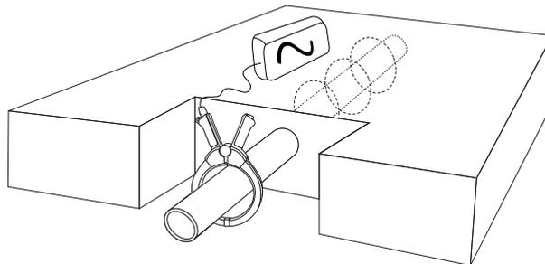
In many situations, it is not possible to gain access to a cable to make an electrical contact. Or if there is, it is not safe to do so. The signal clamp provides an efficient and safe method of applying a locate signal to a cable.
