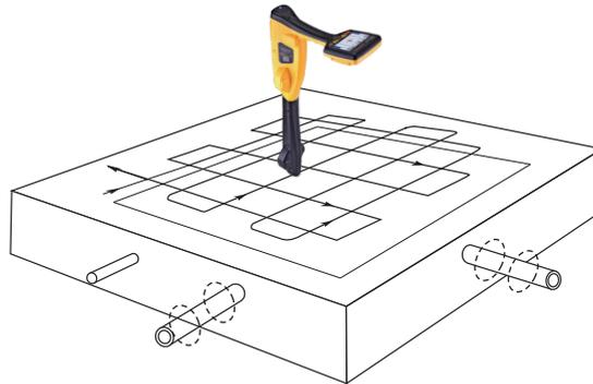
4. Keeping the vLoc3-Cam vertical, walk across the area to be checked keeping the orientation so that the display is pointing to the front. (See diagram above).
