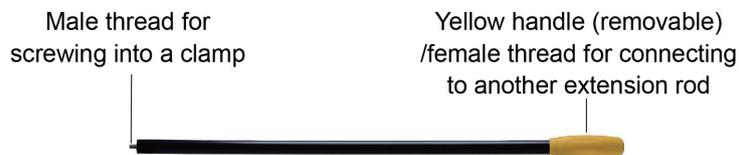
The extension rod is fitted with a 10mm threaded male stud. This male thread screws into the handle of the signal clamp to extend the distance of the clamp. This is helpful in areas with difficult access such as in manholes or overhead cables (not to be used on uninsulated overhead power cables).
