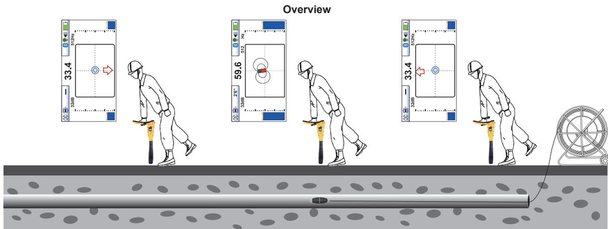
12. Note that when directly over the Sonde, it may be necessary to confirm the position of the Sonde, left to right. To do this move the locator left to right to identify the position of the strongest signal as indicated on the bar graph. At this time the depth to the Sonde will be displayed at the top of the display.
