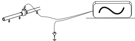
Active locating has the benefit that, unlike passive detecting, the operator is in control of the signals and therefore can be more specific about what line is detected. That is to say active signals can be used for line tracing. Also, passive signals are not always present on a line so using active signals ensures more lines are detected. (For passive locating see section 4.9)
