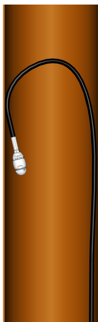
IMPROPER USE: Tool will turn around in large diameter pipe VERY DANGEROUS!
