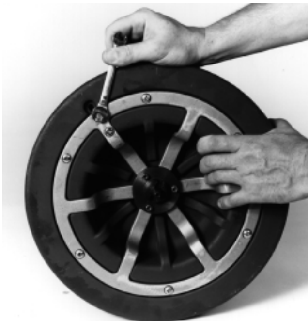
Figure 12 – Loosen Cable Bracket
