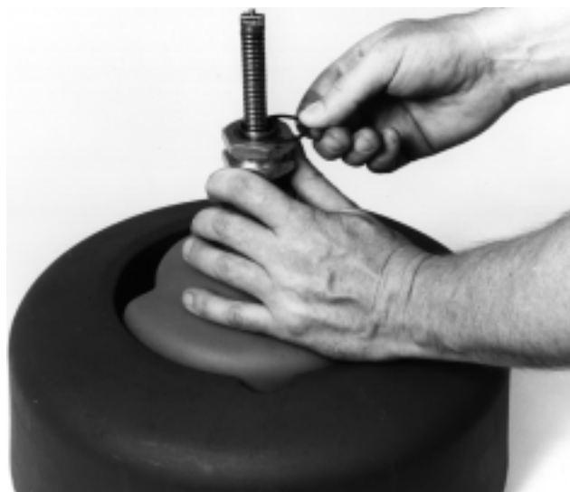
Figure 17 – Reassemble Inner Drum, Front Bracket and E-Clips
