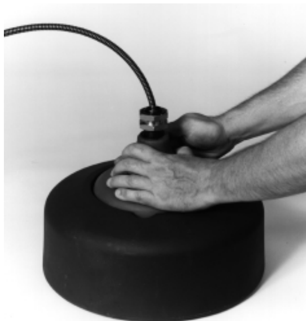
Figure 13 – Removing Cable End
