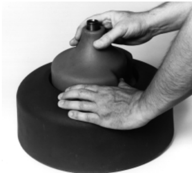
Figure 15 – Removing Inner Drum
