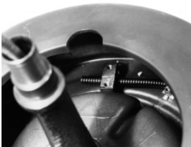
Figure 16 – Position New Cable Under Bracket
